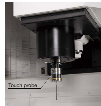
Auto zero offset, auto gauging (radio transmission)
