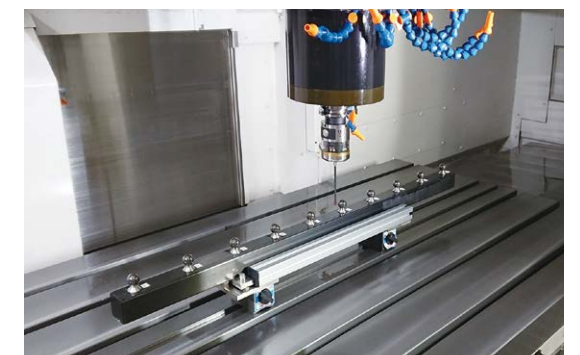
Automatic measurement of ball beam by touch probe
