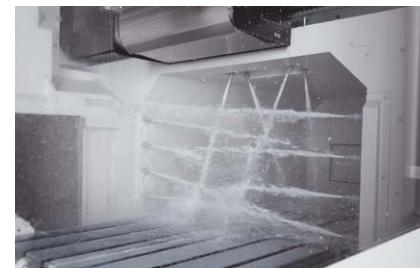
Cross-rail mounted shower coolant (option) wash chips off the workpiece and table.
