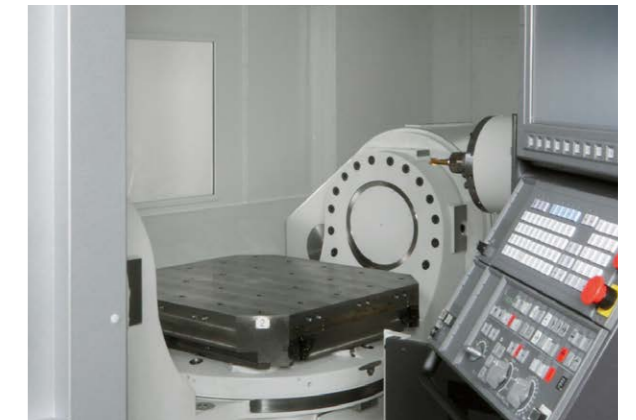
Outstanding access to tools, workpieces · Emphasis on operator visibility and easy confirmation of tool edge and machining portions
