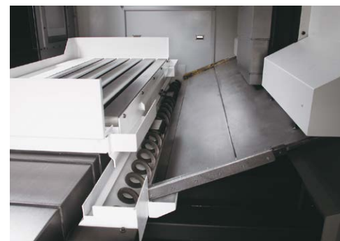
In-machine chip discharge: Coil MILLAC 611VII
