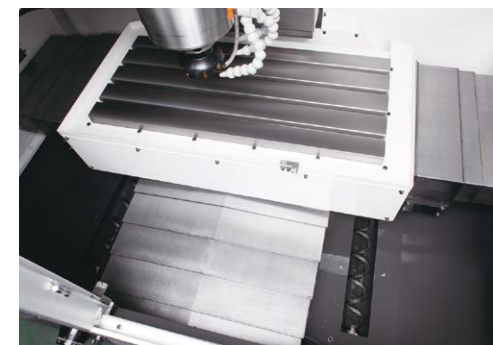
In-machine chip discharge: Coil MILLAC 468VII
