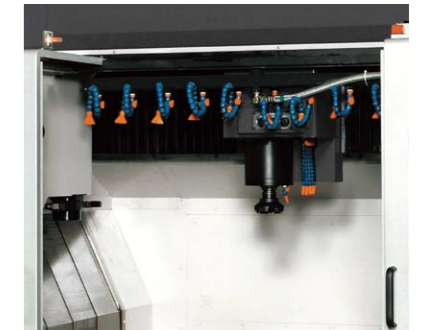
Shower coolant (ceiling)
