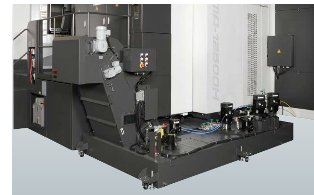
Hinge + scraper (with drum filter) lift-up chip conveyor
